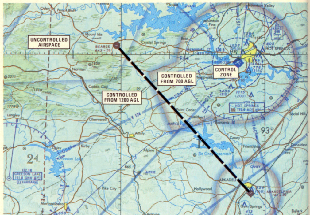
Figure 1. A portion of the Memphis sectional aeronautical chart, illustrating the method of depicting a control zone, controlled airspace having a floor 700 feet above the earth's surface, controlled airspace having a floor 1,200 feet above the surface, and uncontrolled airspace. The limits of controlled airspace are color-coded in magenta and blue. The dark edge of the vignette indicates the limit of controlled airspace, and the vanishing edge the direction of controlled airspace.
